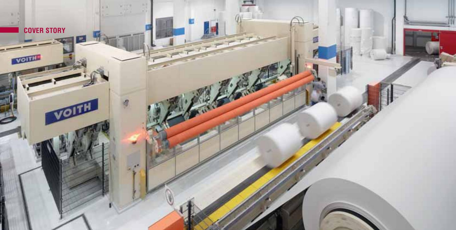
*Fig. 4: The center winding principle of the two VariTop winders ensures good core-winding tightness, an important quality parameter for processing in fast-running printing machines.*
