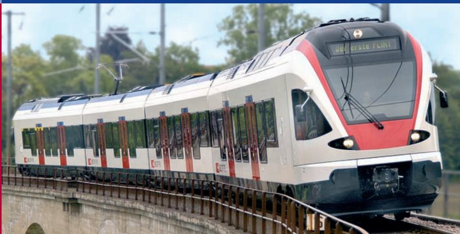
The FLIRT (Fast Light Innovative Regional Train) EMU built by Stadler Rail Group is setting new standards in regional rail traffic with its walk-through passenger area, optimized to a platform height of 550 mm, and its high acceleration capacity. Fitted with 4 x 500 kW TSA asynchronous motors and Voith final drives, the four-car EMU reaches maximum travelling speeds of 160 km/h.
