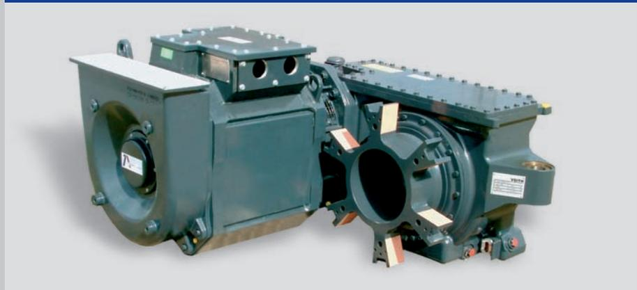
Via a coupling on the primary side, each helical axle drive is connected with an asynchronous motor installed in driving direction. The overhung-mounted rotor shaft of the asynchronous machine transmits the drive torque via a membrane coupling to the helical axle drive. Via the two helical gear stages, drive torque is then transmitted via a single hollow shaft (optimum power curve) and the cardanically acting wedge packet coupling to the
