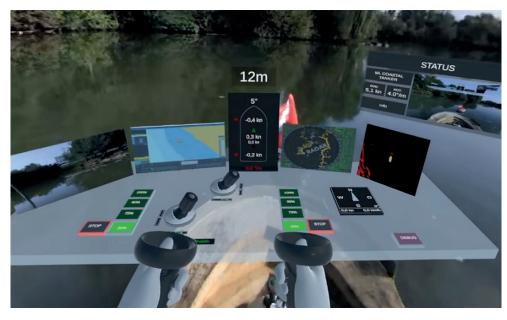
Figure 14: Remote control of model scale tug in AR view developed by Fraunhofer CML
