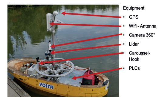
Figure 13: Model-scale remote controlled tug
