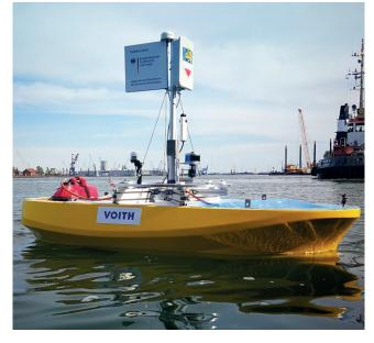
Figure 12: Remote controlled scale model in Rostock harbour
