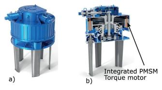
Figure 6: Electric Voith Schneider Propeller, CAD model a) in full view and b) in sectional view.
