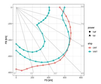
Figure 5: Combined direct and indirect towing mode of remote CRT at 6 kn
