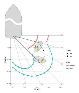
Figure 3: Influence of available power on direct and indirect towing at 6 kn
