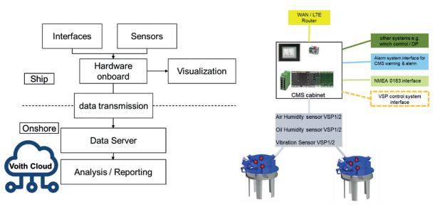
Figure 8: Voith Condition Monitoring System (CMS)
