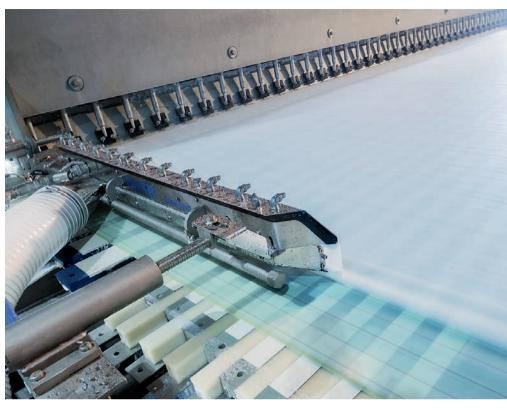
Clean design, easy installation and efficient operation: the unique EdgeExpert concept saves fibers and adds stability.
