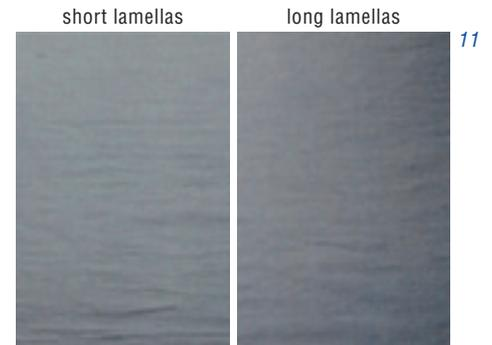
Micro-turbulence in the free jet is mainly created at the end of the nozzle by fluid friction, due to the high acceleration of the flow in this area.
