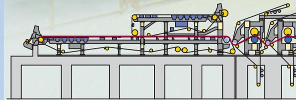
In terms of technology, the new mill is able to clean and fractionate fibers, by separating long from short fibers, in order to treat them differently, without any damage, thus obtaining a higher strength level at lower basis weight. Due to the project modernization level, all contaminants from treatment plants are removed in a solid and compact way. In addition, the noise level and water consumption are reduced, and the plant is ISO 14000 certified.
