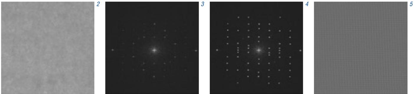
image, in which periodic elements are represented by sharp peaks and other variations by continuous shading. This is followed by interactive filtering of the FFT spectrum and an inverse FFT. This method firstly detects any periodic content in an image over a wide range of frequencies, then allows the periodic and non-periodic contributions of the image to be separated.
