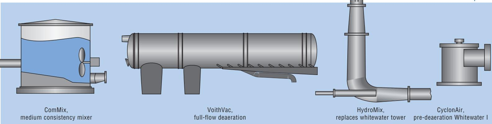
Fig. 1: Components of the Advanced Wet End Process.
