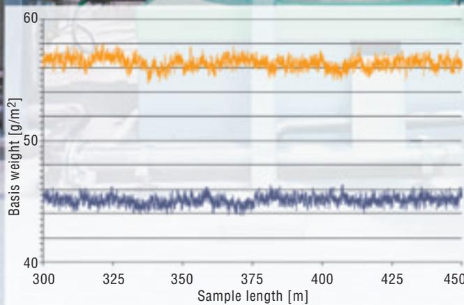
Fig. 5: MD basis weight variations on Kehl PM 2 compared with a conventional approach flow (Boyle Profiler).
