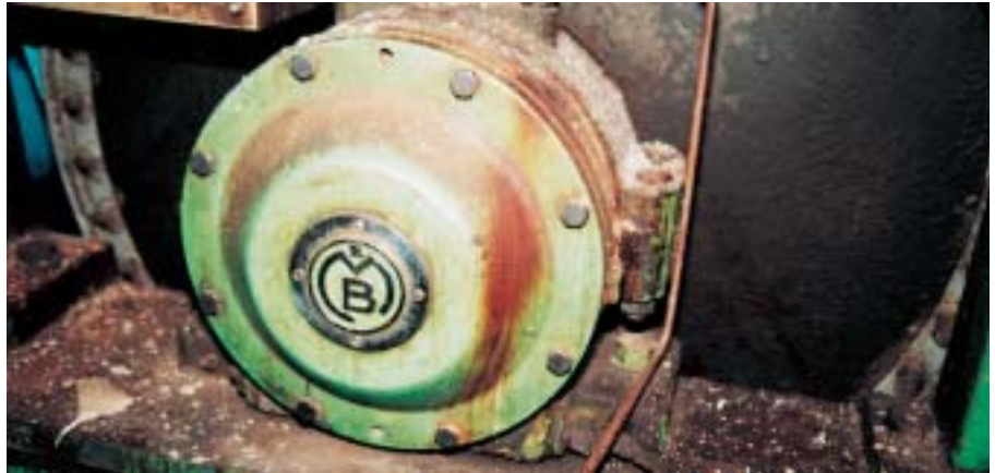
Figs 6, 7 and 8: Three important points for mechanical inspection: roll bearings, doctor moving systems and corrosion on all structural components.
