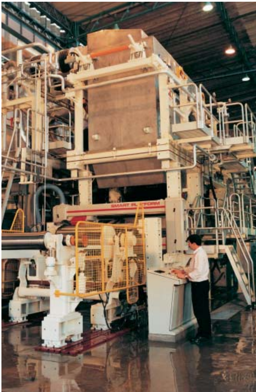
Fig. 10: São Paulo, Brazil: test paper machine for tissue grades with twin wire forming section and crepe cylinder.
