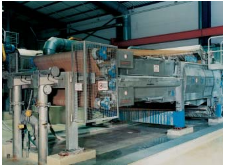
Fig. 6: Disperger with heating screw.
