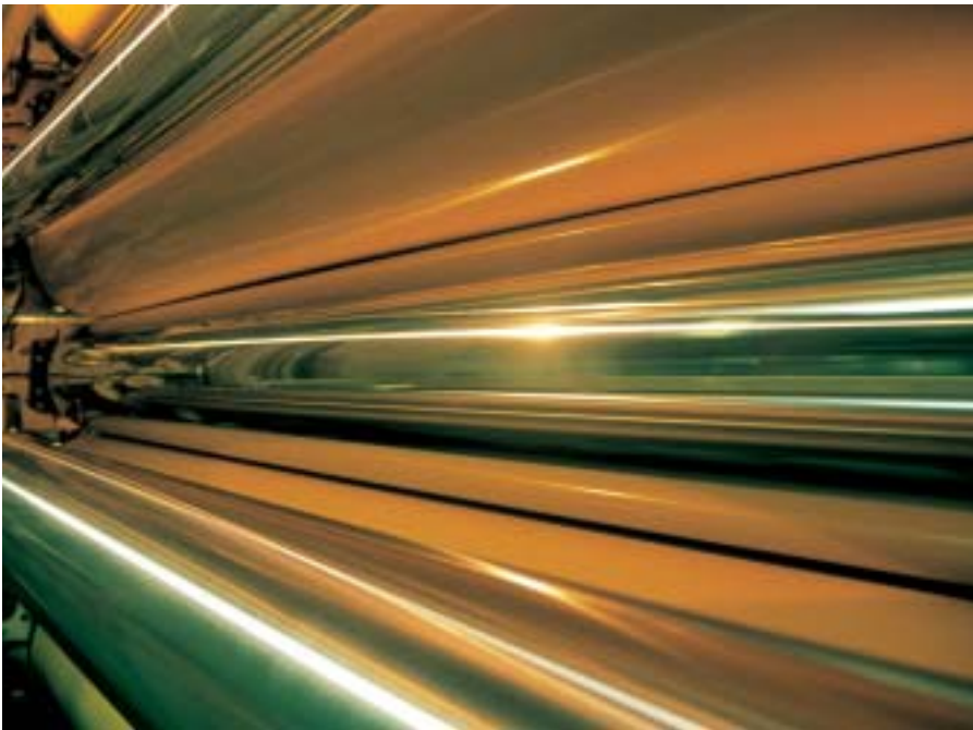
Fig. 7: The calender roll surface smoothness is fully transferred to paper gloss.
