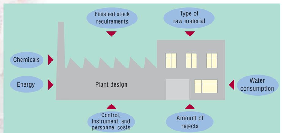
Fig. 1: Factors influencing the design of the plant.
