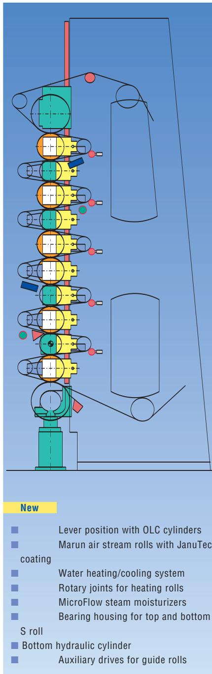
Fig. 1: Different Janus calender lay-outs, 1 x 6 rolls, 2 x 5 rolls, 2 x 7 rolls, 1 x 11 rolls.
