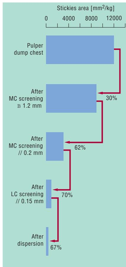
The stickies area in mm<sup>2</sup>/kg is also shown in Fig. 10. Measurement of the stickies area was carried out based on the Haindl-Escher Wyss method. Three process stages are of particular importance for the reduction in stickies area:
