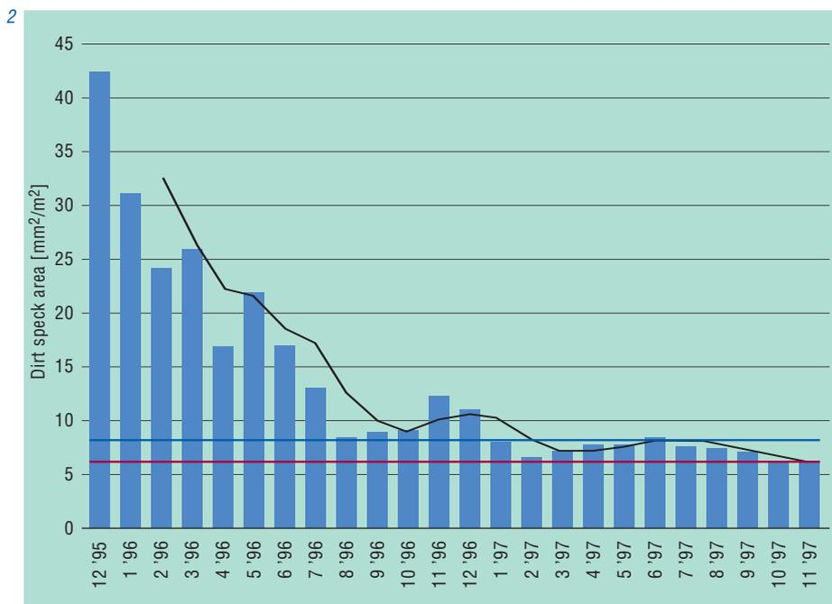
96,000 tonnes. The utilization rate of the deinking plant depends primarily on the amount of deinked pulp used in the paper mill. It requires a considerable learning process for the stock preparation technician and, in particular, for the papermakers, to be able to use a high proportion of deinked pulp without detracting from paper machine efficiency and product quality.
