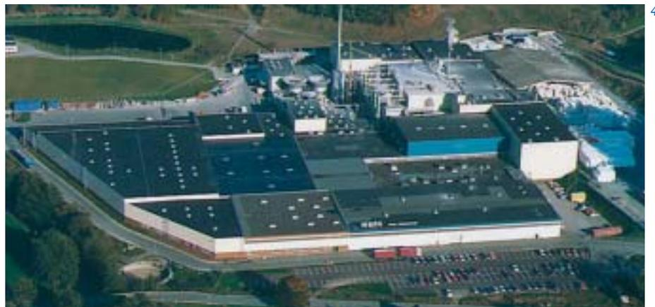
for a speed of 2200 m/min. At the Giershagen mill (Fig. 4) there are two tissue machines and a fourdrinier machine on which towels and crêped papers are manufactured. While the fourdrinier machine has a maximum speed of 920 m/min, speeds of 1600 to 1900 m/min are normal on the tissue machines.
