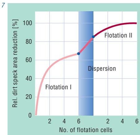
most effective modules, i.e. with flotation and dispersion, is required. With a residual load of 200 ppm and a cleanness target of 10 ppm, the efficiency must be increased by an additional 95%. This corresponds to three additional modules with an individual efficiency of 65% each.
