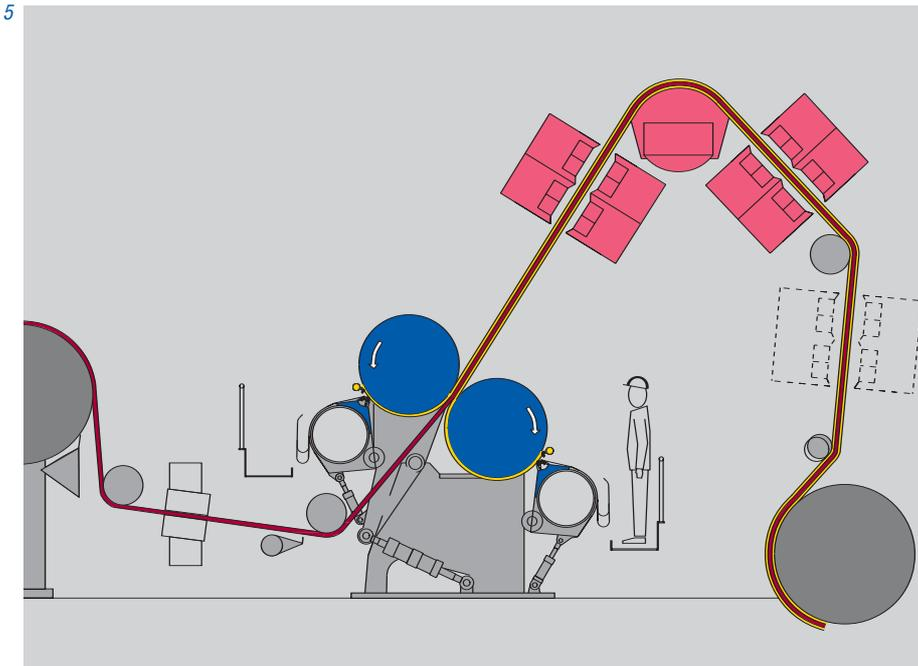
**Concept 2:** For installation into existing paper machines with restricted space conditions:
