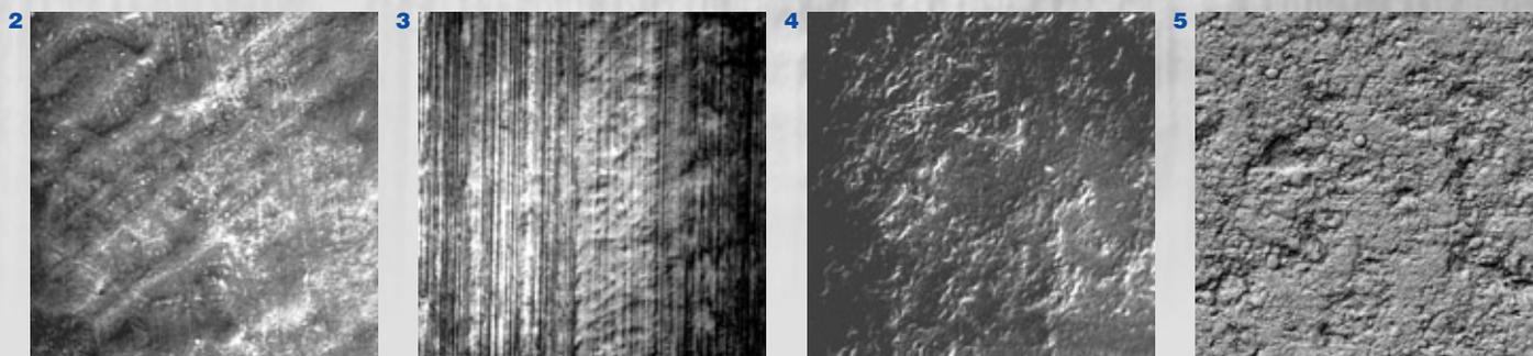
The steel or grey cast iron rolls used in the first supercalenders wore out so rapidly that they soon had to be replaced by chilled cast iron rolls. The impression of such a roll surface in **Fig. 2** clearly shows the roughness due to the relatively coarse iron carbide microstructure.
