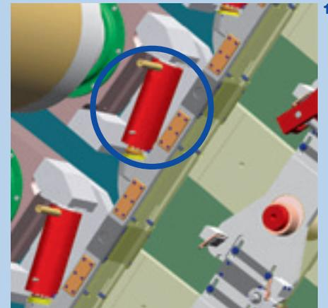
**Fig. 1:** Compensation cylinder.
