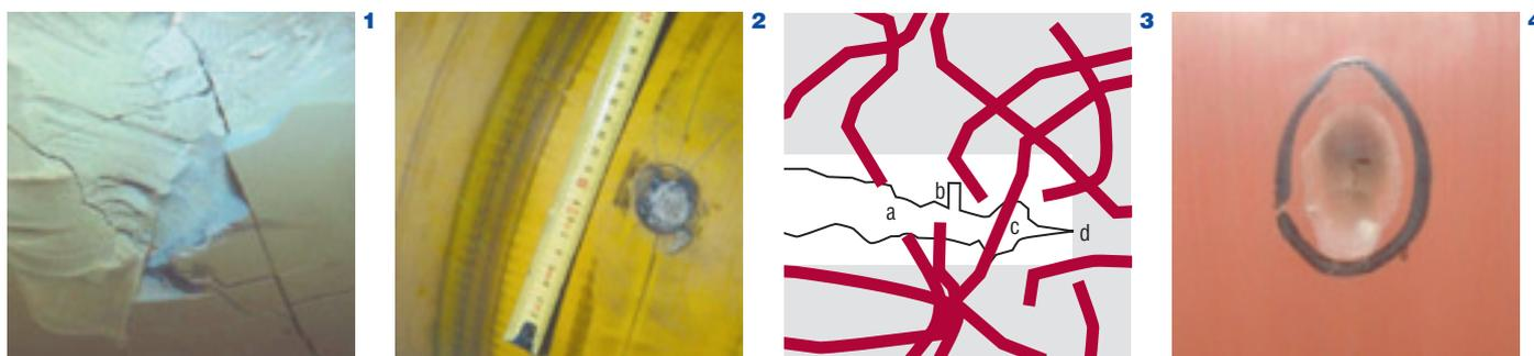
the temperature rise causes cover expansion mainly in the radial direction. This process is repeated with every nip pass. The sum effect of periodic overloading and thermal expansion is a self-energizing cycle, which even might continue after the initial pulse due to roll deposits ceases.
