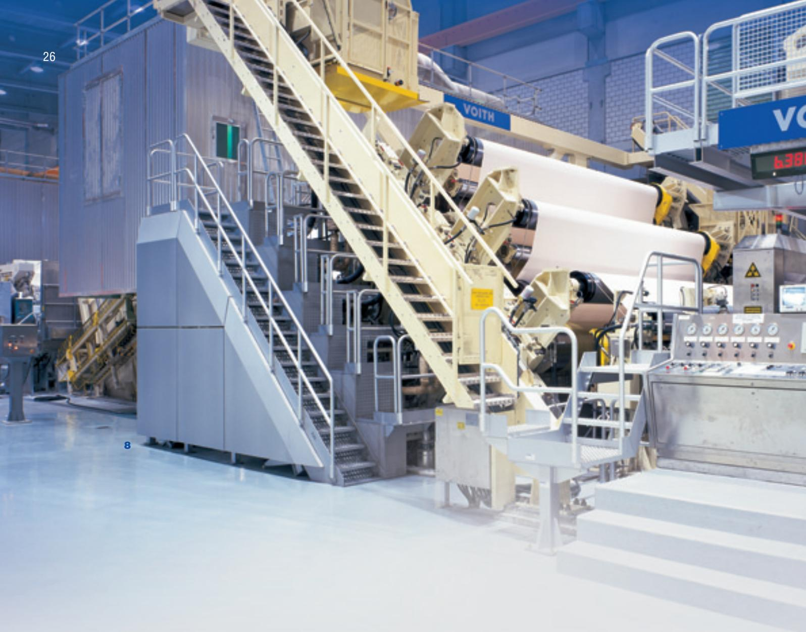
here, up to paper roll diameters of 3,200 mm and with minimal waste, is ensured by a Sirius™ reel system at the end of the line.
