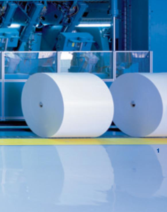
**Fig. 1:** VariTop™ slitter-winder on PM 11 at SCA Graphic Paper, Laakirchen.
