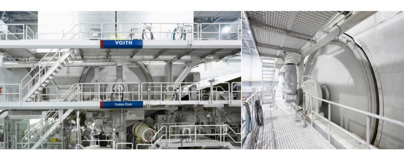
Perfectly coordinated processes and products are necessary to ensure production of high-quality tissue or specialty paper. The dryer section with Yankee cylinder or MG cylinder plays an important role in reaching the required dry content and paper quality. In the drying process, energy is one of the main cost drivers. Therefore it is necessary to equip your dryer section with cylinders that fulfill your technical requirements while using less energy.
