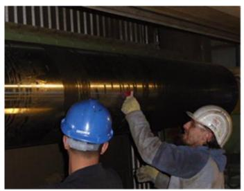
Before the installation of TerraDry PN, cleaning of the chrome-plated steel roll was required during every shutdown.
