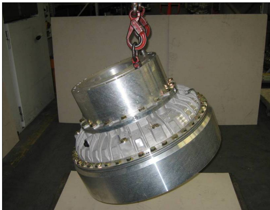
Picture exemplary. Shown lifting of a T-coupling
