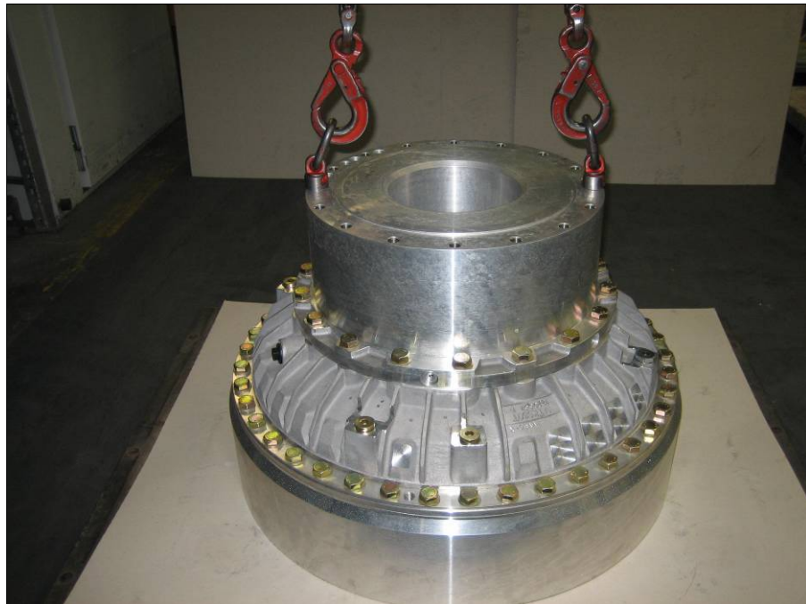
Picture exemplary. Shown lifting of a T-coupling
