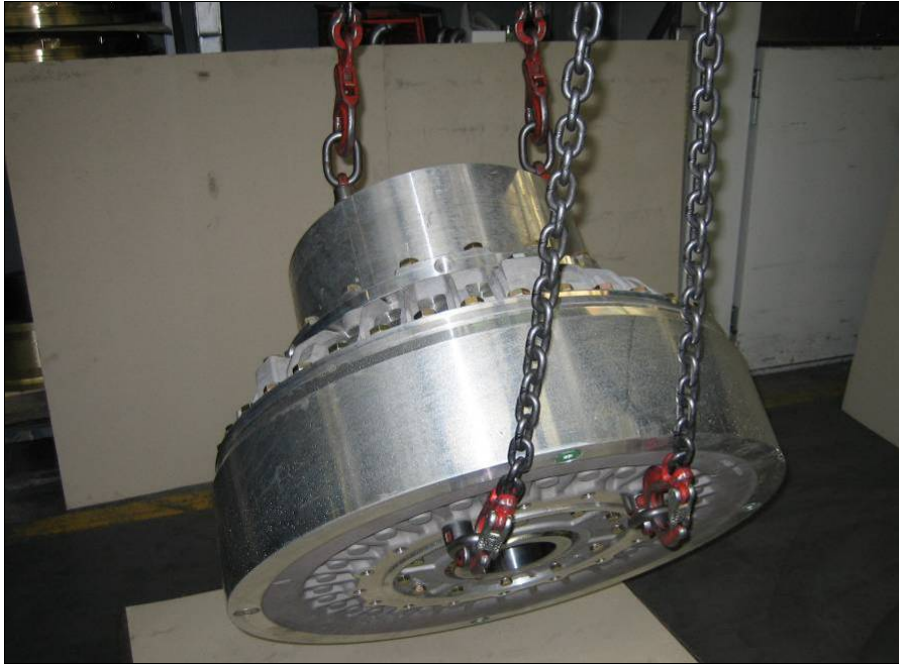
Picture exemplary. Shown lifting of a T-coupling
