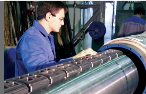
The axle of a Nipcorect™ roll is inserted accurately into the roll sleeve.
