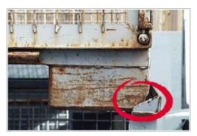
→ The wire mesh is so torn that the wire ends extend to the inside or outside, (one missing mesh per side is allowed),
