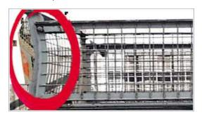
→ The hinged front panels (upper and lower) are immovable or deformed in a way that the pallet cage cannot be closed anymore,
