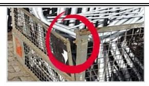
→ The floor frame or the pallet feet are so heavily bent that the pallet cage no longer stands firmly on 4 feet
