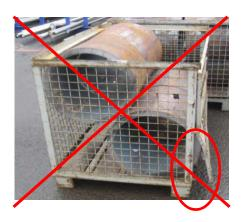
The pallet cage is too heavy and cannot be stacked anymore, the pallet cage is pressed apart. The material projects the pallet cage.
