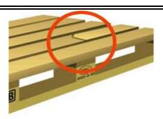
ightarrow A log is missing or split in a way that more than one nail is visible,
