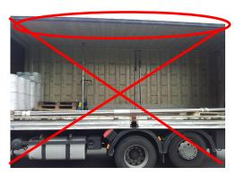
The material cannot be unloaded from the top. The lorry must be accessible from the top.
