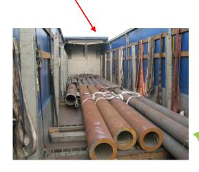
The material must be unloaded from the top by crane, a slip must already be placed around the pipes.
