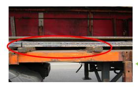
Gaps must be left between the individual layers by means of timber so that the forklift can unload, external material must not be present on the sheet metal.
