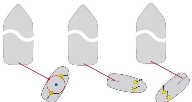
Figure 4: CRT combination of direct and indirect towing
