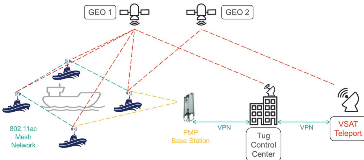
Figure 2: Data transmission concept designed by MediaMobil (source MediaMobil)
