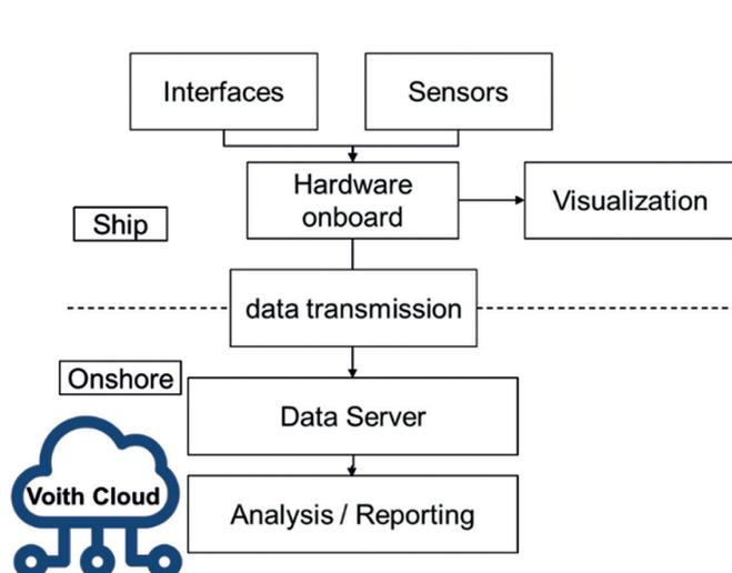
Figure 8: Voith Condition Monitoring System (CMS)
