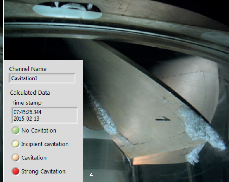
1 + 2 Examples of cavitation damages
