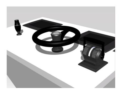
Functional model of the new vessel propulsion control system for Voith Schneider Propellers and Voith Radial Propellers
