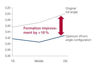
The individual adjustment of every single VForm hydrofoil results in a significant improvement in formation.
