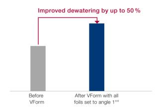
An optimization of the VForm hydrofoil setting leads to a significant increase in dewatering capacity. In tests, dewatering was improved by up to  $50\,\%$ .
