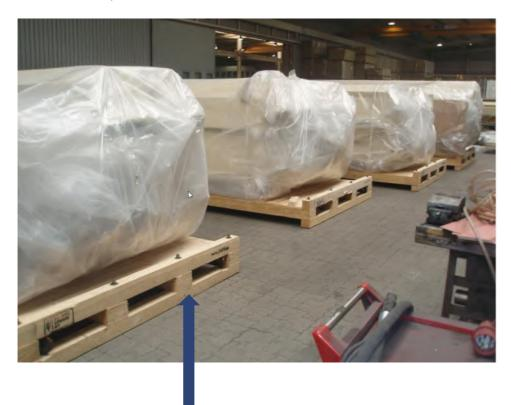
For ocean transport, the crate bottom must be supported as a wood transport slide for moving into the container.
