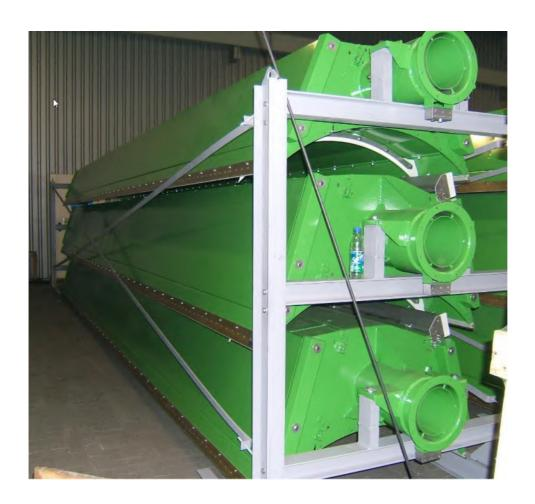
**Figure 2**: Irrespective of whether land/air or sea freight, the boxes, including the steel frame, must be packed with a VCI foil.
