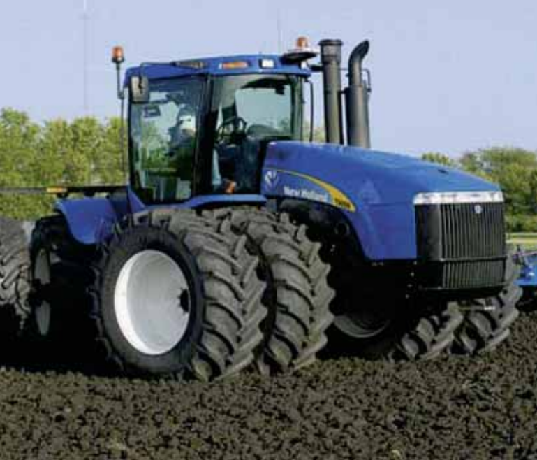
Off-road application in CNH 4x4 tractor with Iveco 13 TCD Cursor engine
