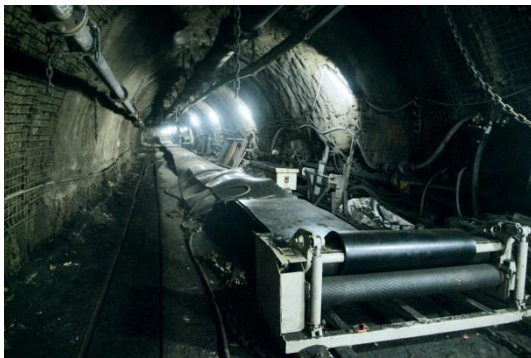
The H2 belt conveyor of RAG during belt replacement. (Photo: RAG)
