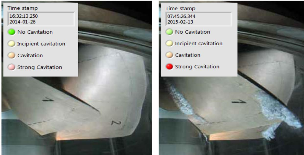
Fig. 4. Operating points without cavitation (left side) and strong cavitation (right side)
