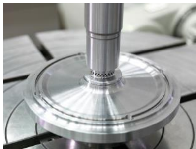
Voith Hirth coupling connecting the shaft and impeller
