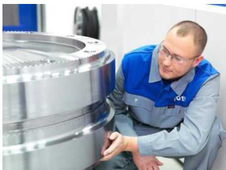
Gas turbine disk array with Voith Hirth couplings
