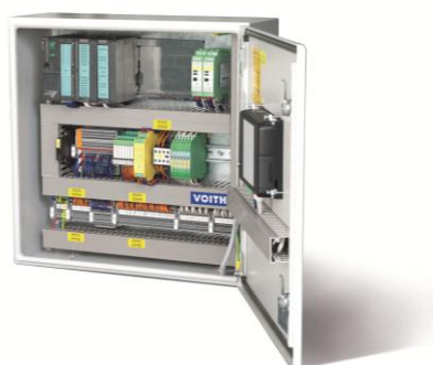
Figure 2: The digital TurCon DTm steam turbine controller from Voith is fully equipped with all the relevant components – no need for any additional equipment. The result: reduced total cost of ownership for the operator. The wide array of TurCon DTm components includes an industrial CPU, I/O modules, speed measurement system, safety or TRIP relays, isolation amplifiers and a touchscreen display.
