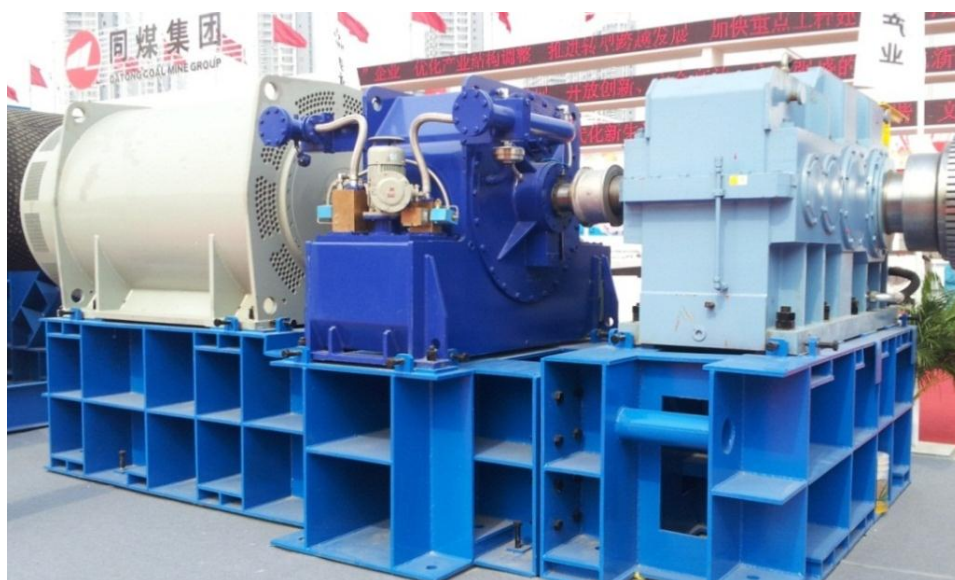
Figure 1: Powerful 866 TPKL fluid coupling from Voith protects the belt conveyor as well as the drive components against damage and prevents unplanned downtime.
