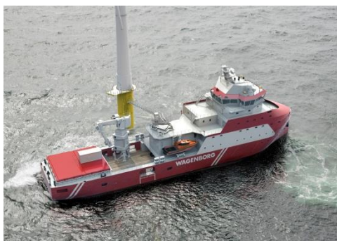
Equipped with two VSPs and two VITs, the new W2W vessel can be positioned to the meter next to platforms and wind turbines
