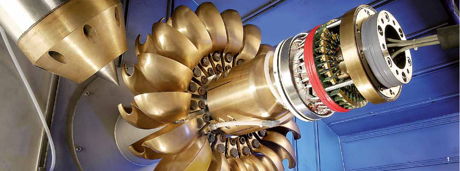
Cover picture Machined bucket backside, Workshop, St. Pölten, Austria
