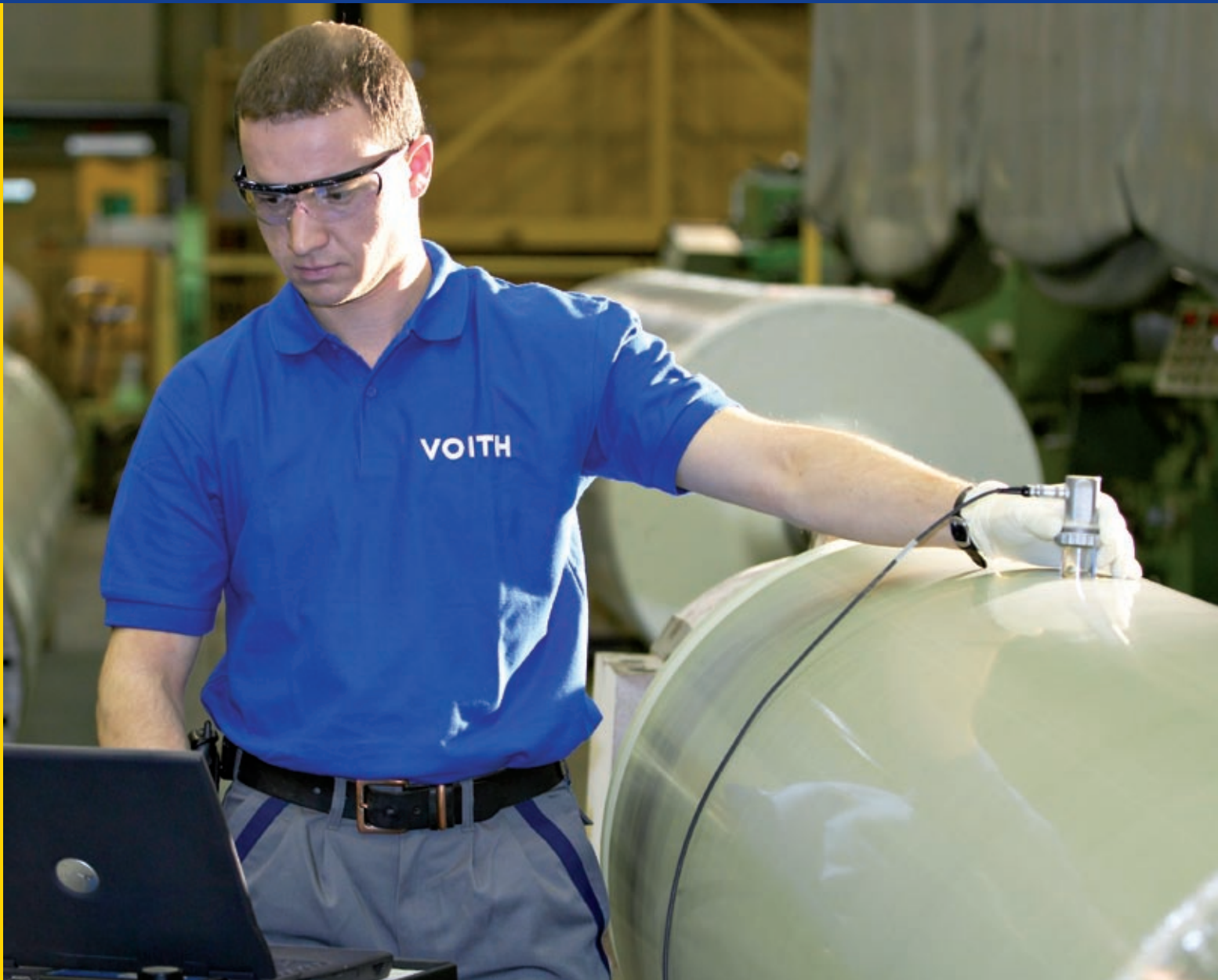
RollCare: 辊子面层的超声波检验
