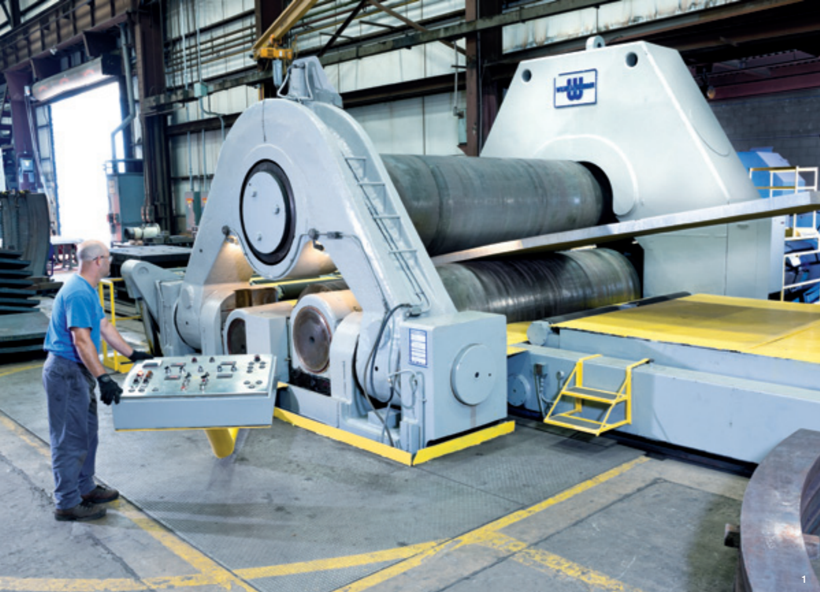
1 WilhelmsburgerRolls can shape plates as thick as 13 inches
