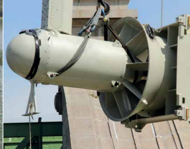
1 Typical Power Plant Arrangement with StreamDiver 2 First StreamDiver Prototype Turbine
