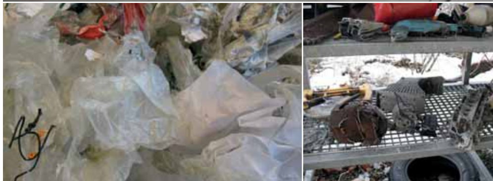
Fig. 6: Normal contaminants, which the IntensaMaXX separates and which are removed from the downstream drum screen.
