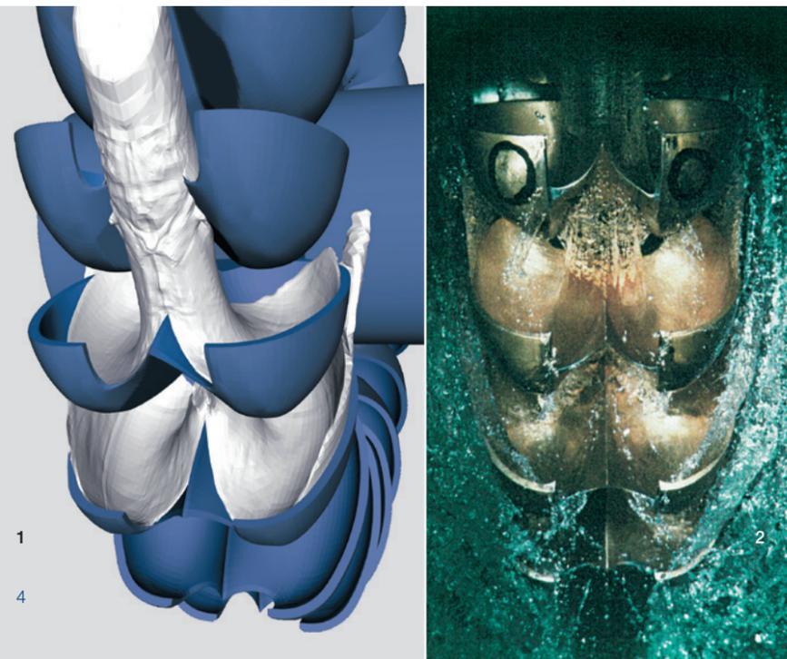
1 Simulated flow through Pelton runner
