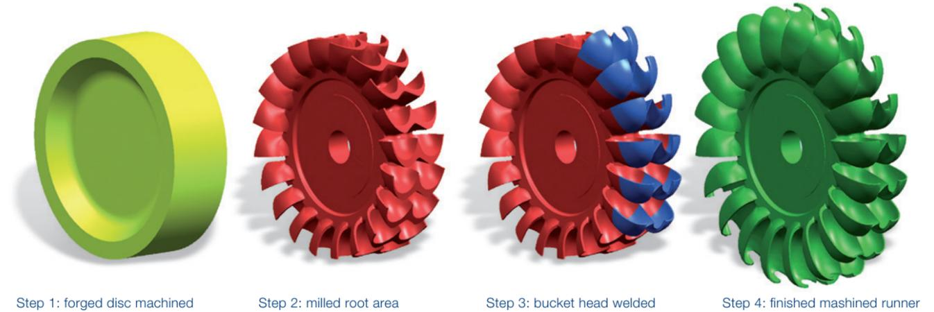
Step 1: forged disc machined      Step 2: milled root area      Step 3: bucket head welded      Step 4: finished mached runner
