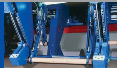
Cores being put onto the rewind chucks of the rewind stations
