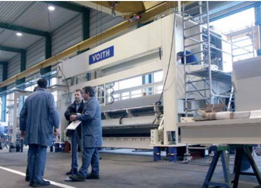
The main functions of the Voith Paper winders are tested together with the customer during factory pre-assembly.
