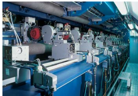
Slitter section – slitter positioning by two independent belts
