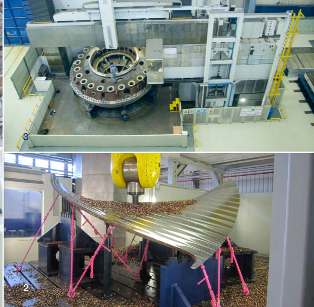
1 Shaft Manufacturing Cell 2 5 Axis Milling Machine 3 Vertical Machining Center
