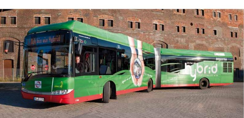
In fact, thanks to the supercaps, the diesel engine is protected somewhat, while the capacitors themselves are entirely maintenance-free. To top it off, particulate emmission is reduced by up to 90% compared to conventional diesel vehicles, carbon dioxide emissions are cut by 30% and the discharge of nitrogen oxides is lowered by almost 40%.
