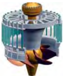
Schematic view of a minimum gap runner Kaplan turbine
