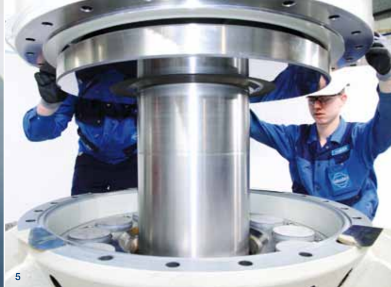
4 Assembled thrust bearing pads
