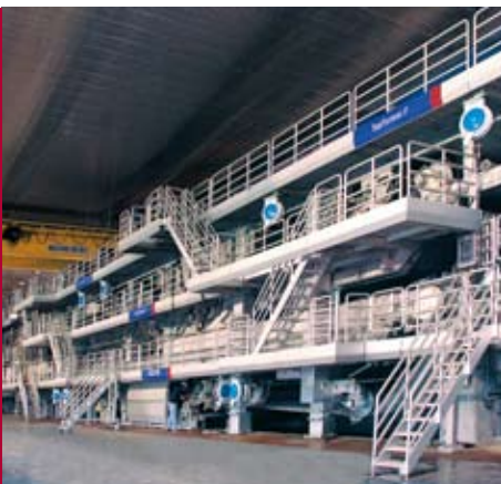
Fig. 1: On multi-ply cardboard machines, measurements can be made on the different headboxes.
