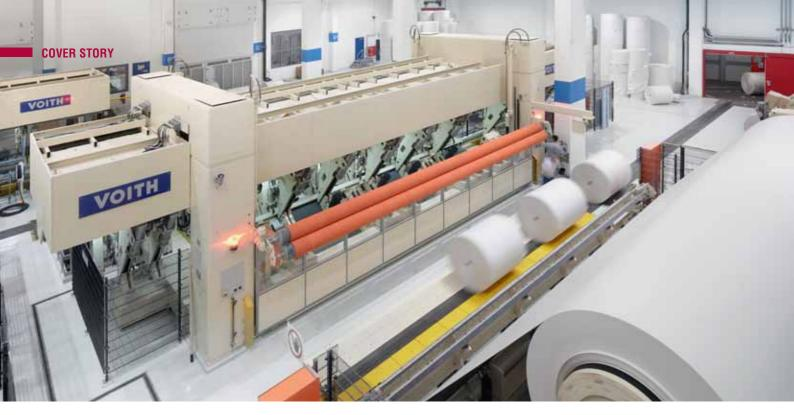
Fig. 4: The center winding principle of the two VariTop winders ensures good core-winding tightness, an important quality parameter for processing in fast-running printing machines.
