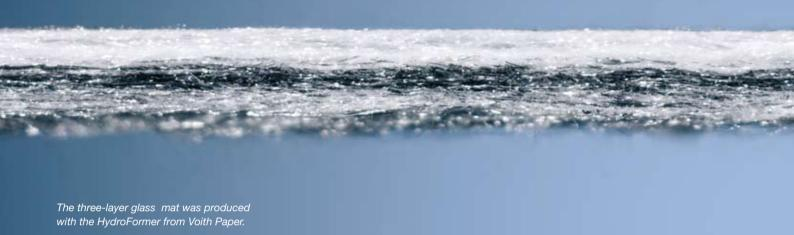
Glass fiber mats are used as the base material for floor coverings, asphalt shingles and asphalt rolls, among other products. There are older glass mat machines operating in the width ranges of 2 to 5 meters. But to achieve higher production capacities the latest installation is the largest glass mat machine in the world. The formation width of the new machine
