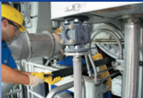
Voith Paper Rolls service technician changing doctor blade
