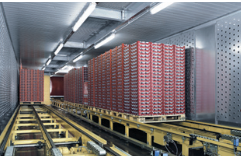
Double acting cooling tunnel (interior view)
