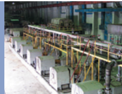
View of the deinking lines with old refiners prior to rebuild
