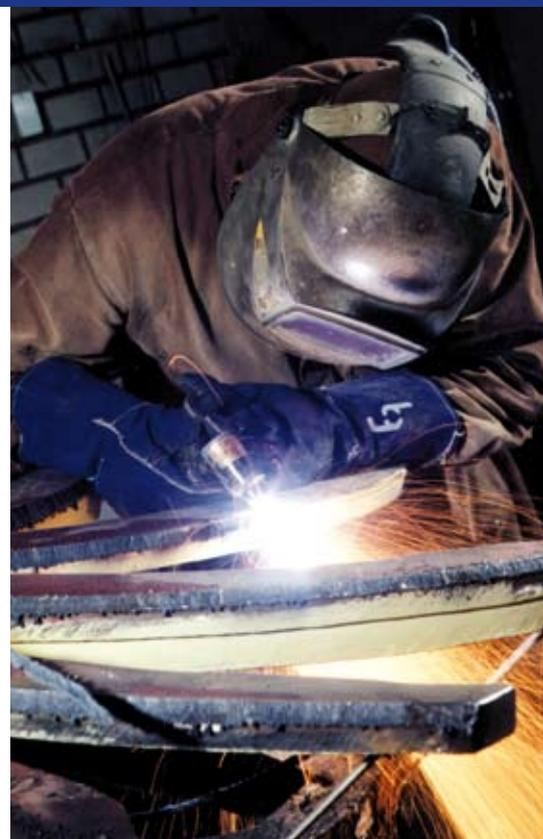
*In depth knowledge from welding technology and materials is required to bring the rotor back to its original design geometry.*
