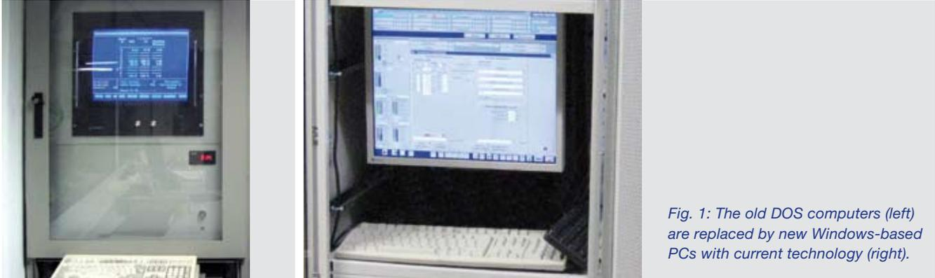
*Fig. 1: The old DOS computers (left) are replaced by new Windows-based PCs with current technology (right).*
