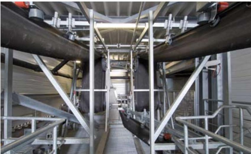
*A closed pouch belt conveyor also allows fuel transport on complicated stretches.*
