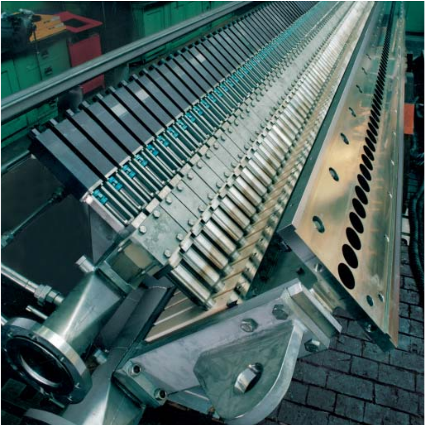
Fig. 4 ModuleJet mixing units.
