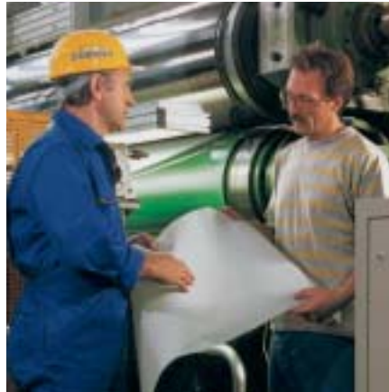
Fig. 11: Final inspection of a remachined calender roll after polishing.
