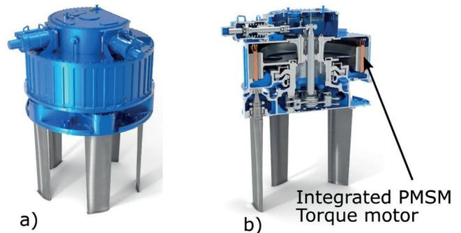
Figure 6: Electric Voith Schneider Propeller, CAD model a) in full view and b) in sectional view.
