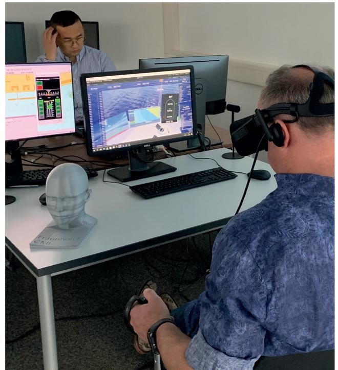
Figure 9: Tests of VR based remote control station connected to ship simulation
