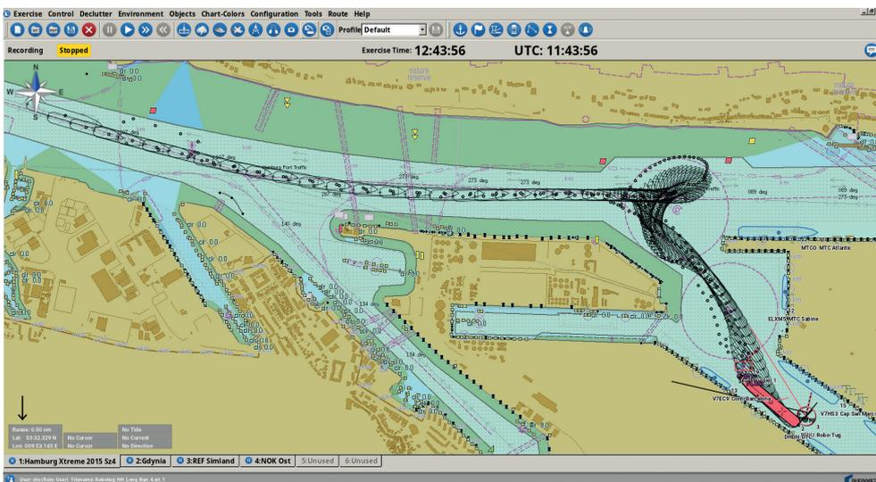
Figure 11: Simulation of tug assistance at MTC
