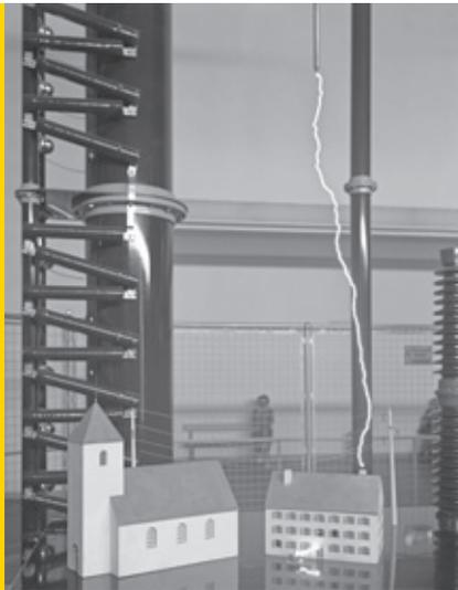
*Lightning model in the high-voltage apparatus.*
