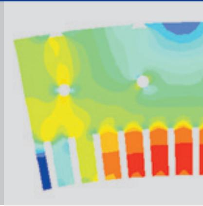
Figure 6: Magnetic induction in the stator core lamination.
