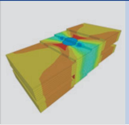
Figure 10: Nonlinear stress-strain analysis of a periodic segment of a rotor rim for homogenized FE analysis.
