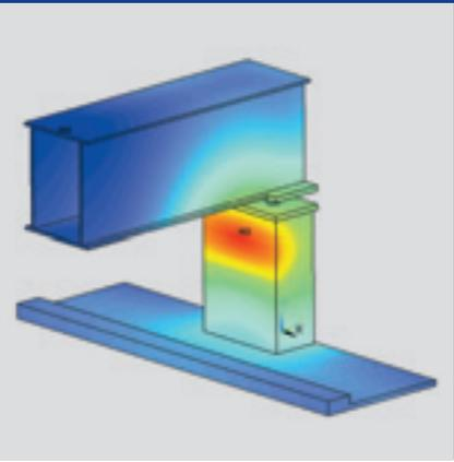
Figure 7: Temperature of surrounding steel components (here: stator frame neck and bracket) due to eddy current heating.
