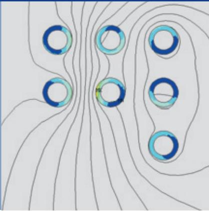
Figure 5: Power loss density in circuit rings and flux lines in surrounding air.
