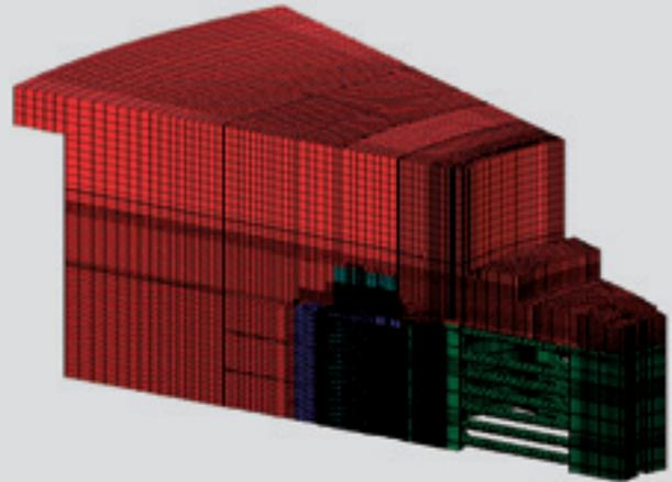
Figure 2: Fluid meshed for flow and thermal analysis.
