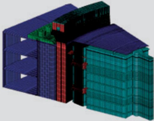
Figure 1: Solid geometry meshed for thermal analysis.
