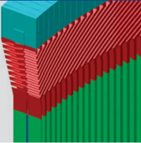
Figure 3: Prescription of homogeneous losses on four different parts of the stator winding.
