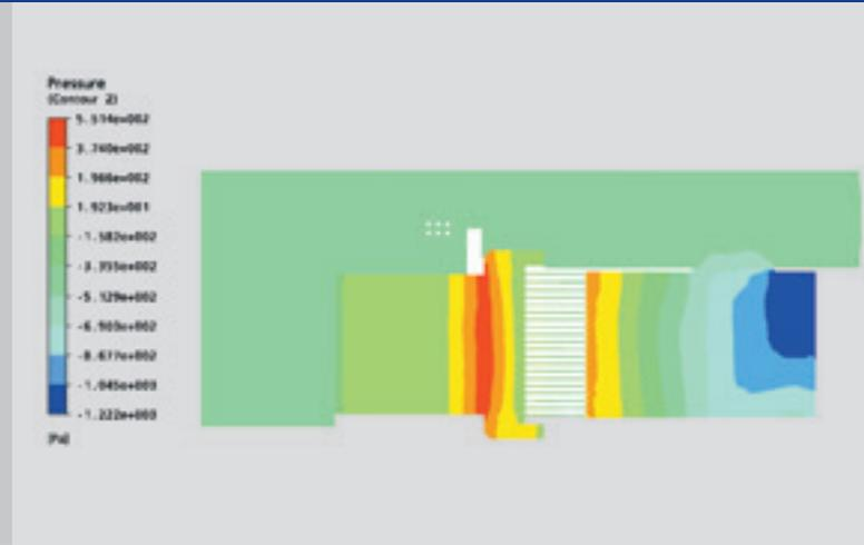
Figure 10: Pressure gradient in section.
