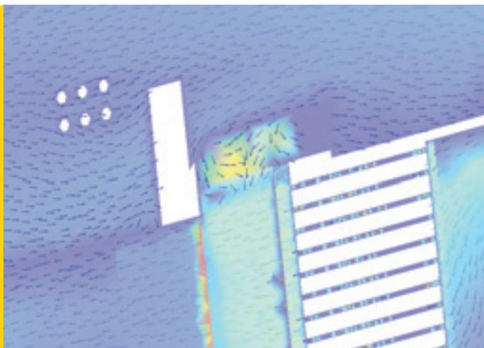
Figure 8: Velocity vectors with recirculation. This is a 3D vector field plot showing the flow of air through the same mechanical structure as in Figure 7. The flow is depicted as a series of blue and green arrows, but it shows significant recirculation and turbulence, particularly in the upper regions of the structure, indicating a more complex and less efficient flow path compared to Figure 7.
