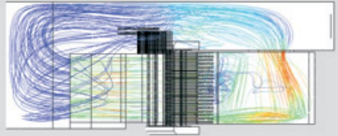
Figure 12: Stream lines (side view).
