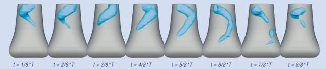
Calculated vortex rope at different times.
