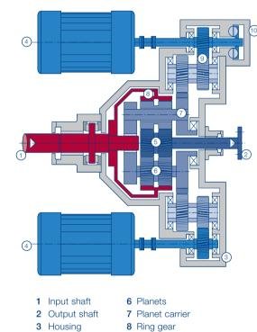
4 Servo motors 9 Helical gears
