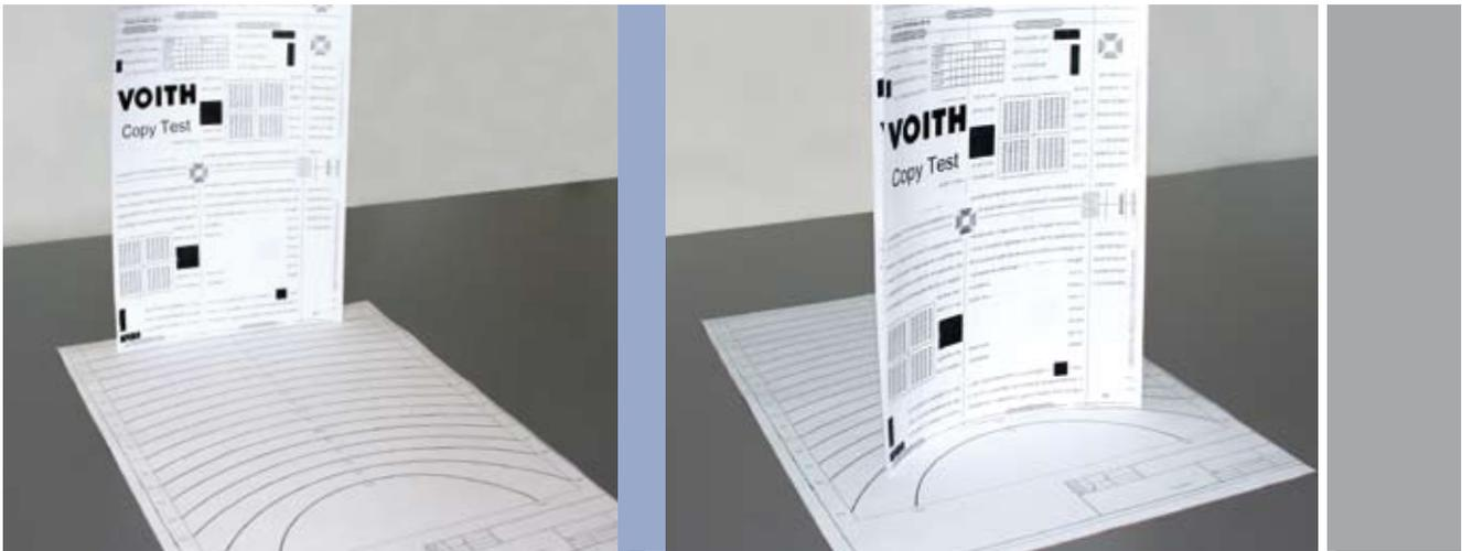
The quality of copy paper is revealed during the copying test. The sample produced with ParaSlice (left) shows a noticeably reduced deformation in comparison to conventionally produced paper.
