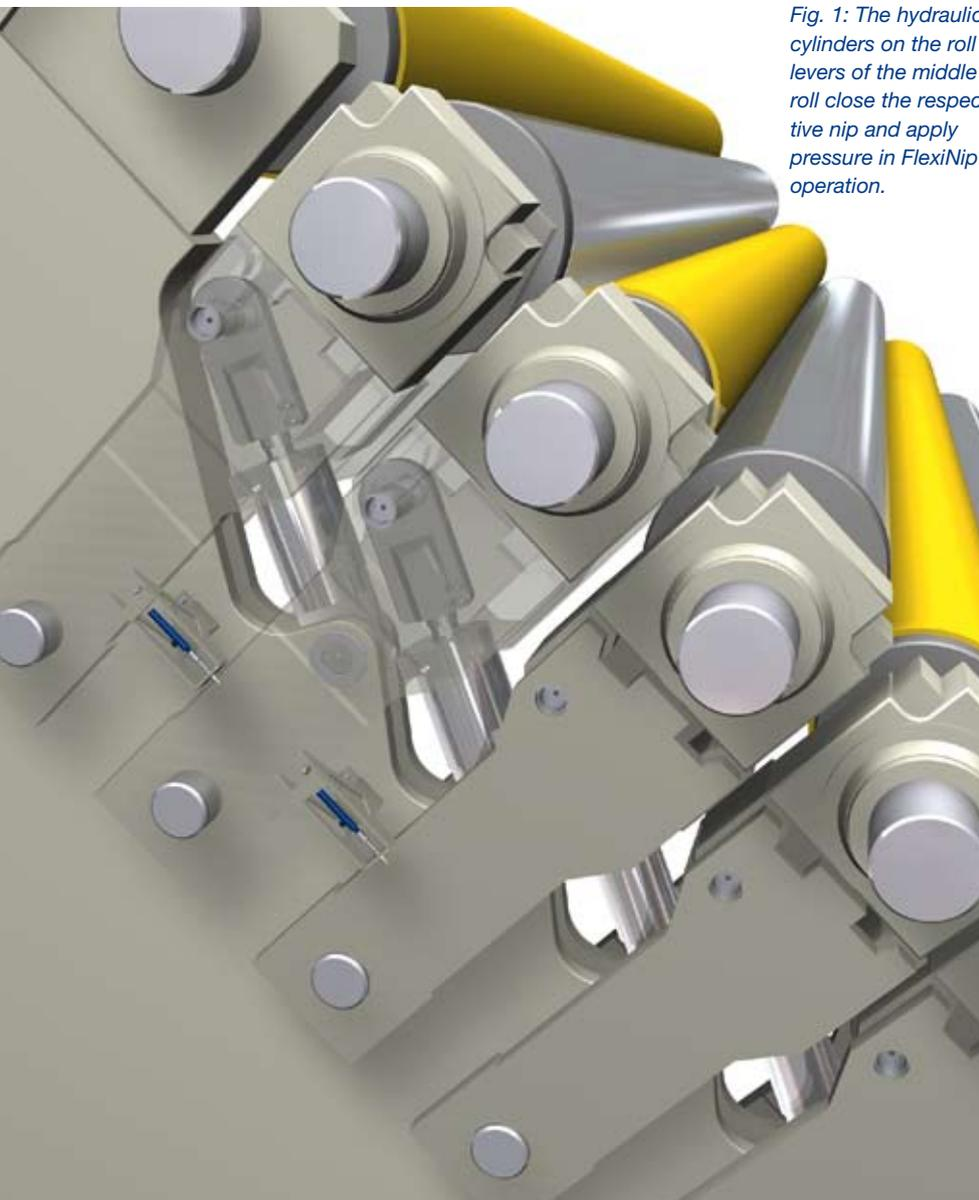
*Fig. 1: The hydraulic cylinders on the roll levers of the middle roll close the respective nip and apply pressure in FlexiNip operation.*
