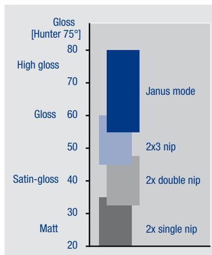
Fig. 7: Quality ranges made possible by FlexiNip.
