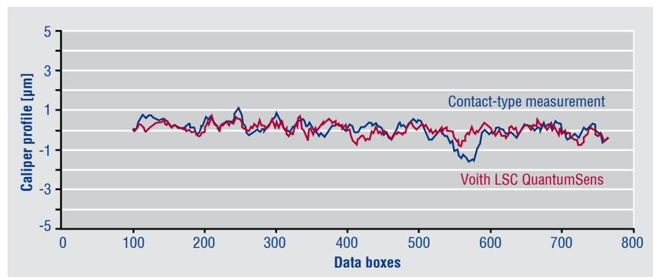
*High accuracy: The new Voith LSC QuantumSens also impresses in a direct comparison with conventional, contact-type caliper measurement.*
